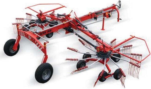
Surmak STR 22 is high performance double rotor central delivery hay rakes offer working widths up to 8.30m.
